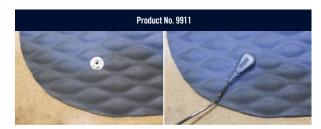
**Heel Grounders** are made for workers wearing rubber soles and other insulating shoes. They allow static electricity to pass around the shoe into the ESD matting. Fasten the Heel Grounder to the heel of the shoe with the Velcro and allow the fabric strip to touch the sock or skin for best performance.
